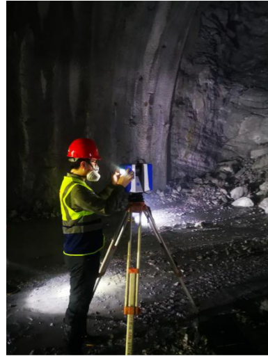
图5 三维激光扫描系统现场作业照片 Fig.5 Schematic diagram of on-site operation of 3D laser scanning system
